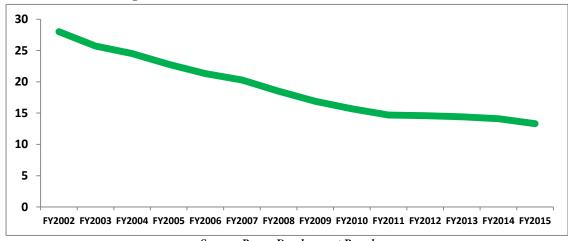
Figure 5.7: Transmission and Distribution Losses (%)
