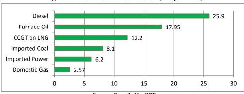
Figure 5.10: Unit Cost of Generation (Tk./per kWh)
