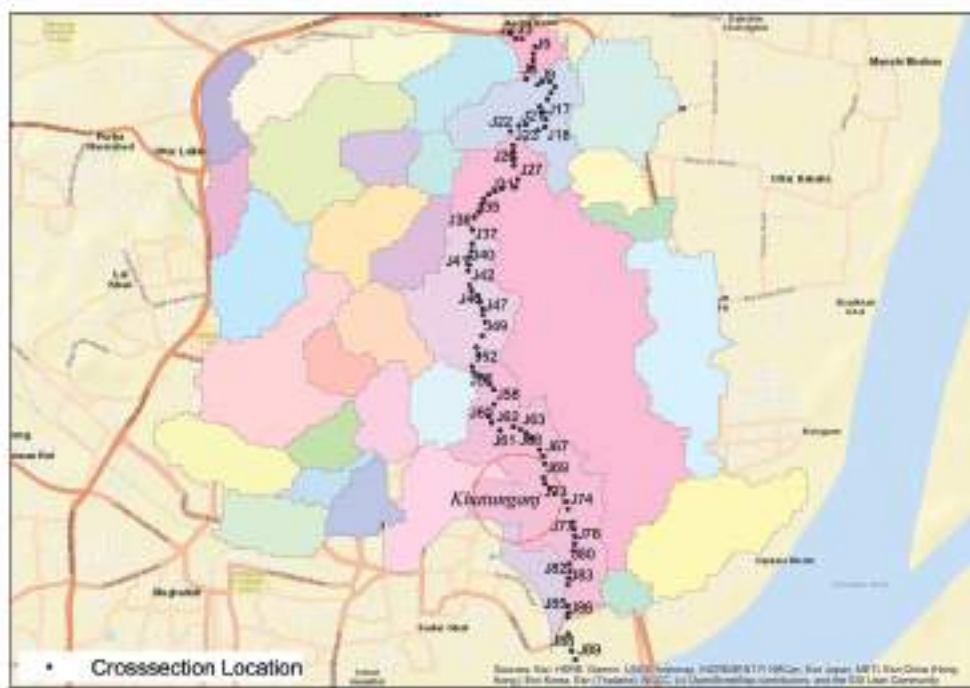
Figure 32: SWMM model setup showing the nodes and junctions (Source: Model setup by Authors)
